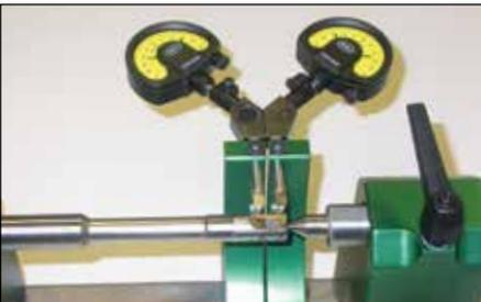
3. Rotate and position the insert against indicators.
