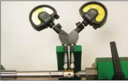
1. Place the reamer between fixture's centering pins.
